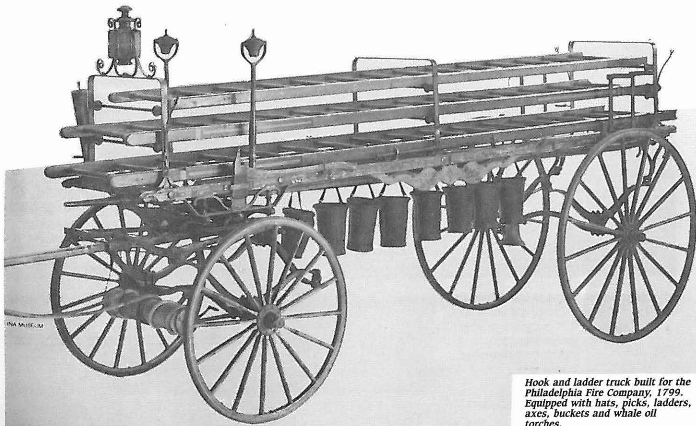
***Hook and ladder truck built for the Philadelphia Fire Company, 1799. Equipped with hats, picks, ladders, axes, buckets and whale oil torches.***
